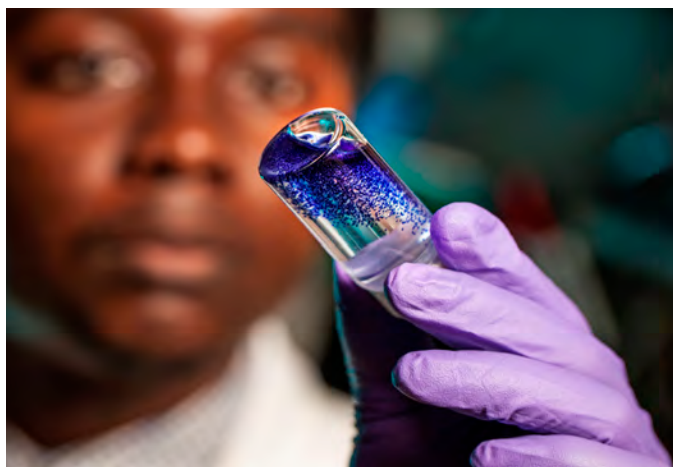
Novel LLNL microcapsules can be used to capture carbon dioxide from coal or natural gas-fired power plants, as well as industrial processes.
