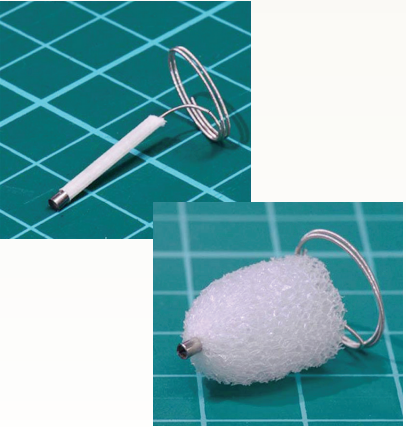
A compressed shape-memory-polymer foam is delivered by catheter to an aneurysm sac within the brain. Once it is activated by temperature change, the foam expands to match the sac’s contours.
