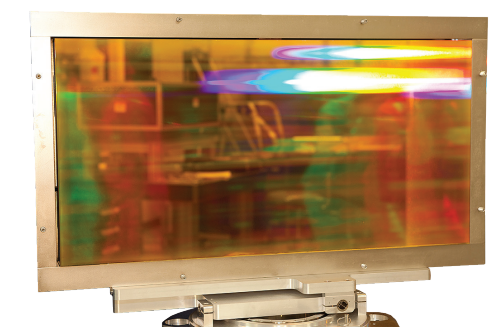
LLNL's Multilayer Dielectric Grating enables the use of higher power lasers by combining separate laser beams into a higher-power single beam. It thus reduces heat and protects laser optics from damage.
