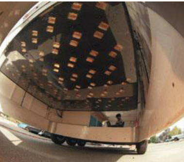
An array of MIR sensors were incorporated into the HERMES bridge inspection trailer in an ultrawideband-based non-destructive evaluation system. By driving the trailer over a bridge at 55 mph, a 3D image of the bridge deck’s structural integrity is created without closing the bridge to traffic.
