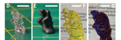
A miniature representation of Auguste Rodin's "Thinking Man" volumetrically printed using computed axial lithography
