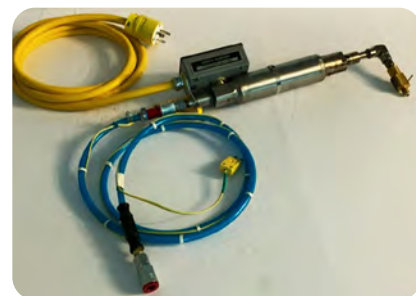
This versatile cold spray control unit allows precise control of gas temperature and pressure, as well as additional in-line diagnostics during the spray process.
