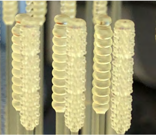
Swabs were 3D-printed at LLNL from a biocompatible, surgical-grade resin and tested in the Laboratory’s Advanced Manufacturing Laboratory.
