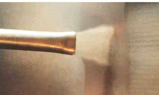
Strips of p- and n-type thermoelectrics (grey ridges) deposited on the outside of a copper pipe, forming a basic thermoelectric generator to harvest waste heat radiated from the pipe’s contents.
