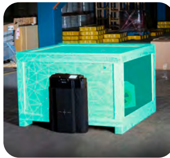
MC-15 is portable, weighs 47 pounds, and is faster than any other available neutron multiplicity detector. In addition, it requires little training to operate.
