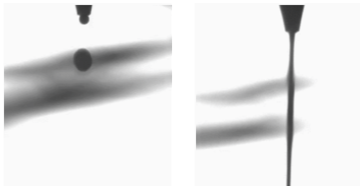
The Livermore LMJ machine offers two printing modes: drop-on-demand (DoD) mode (left), which produces discrete droplets ejected from a 100-micrometer-diameter nozzle (top), and continuous stream mode (right), which is faster than the DoD mode but offers less resolution.
