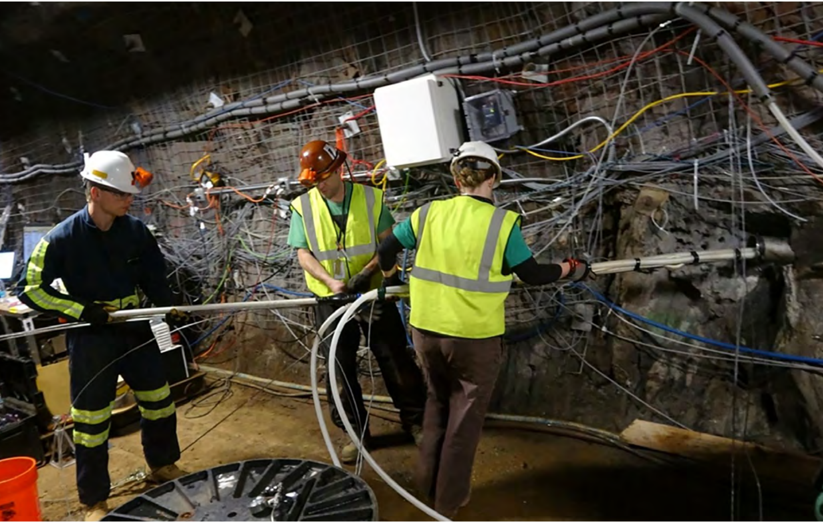
EGS Collab team members work together to add instrumentation for monitoring water injection through the borehole.
