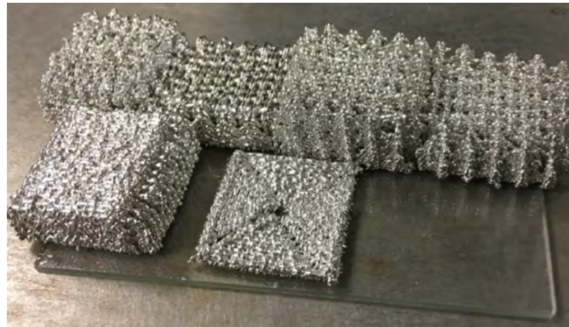
LMJ-manufactured tin parts (all measuring about 3 centimeters to a side) are examined using a combination of roughness, density, and x-ray diffraction measurements. The parts' microstructures have shown minimal stored strain or deformation and exhibit characteristics identical to metal parts produced by conventional machining or casting.
