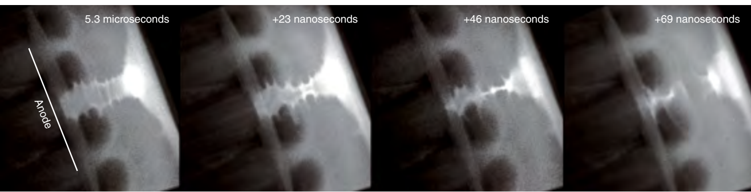
In this image of visible light emission from the pinching plasma discharge, a dense plasma focus (DPF) produces a plasma sheath that pinches, over the course of tens of nanoseconds, eventually becoming unstable and producing an energetic ion beam. The ion beam’s bombardment of a dense plasma target produces neutrons.
