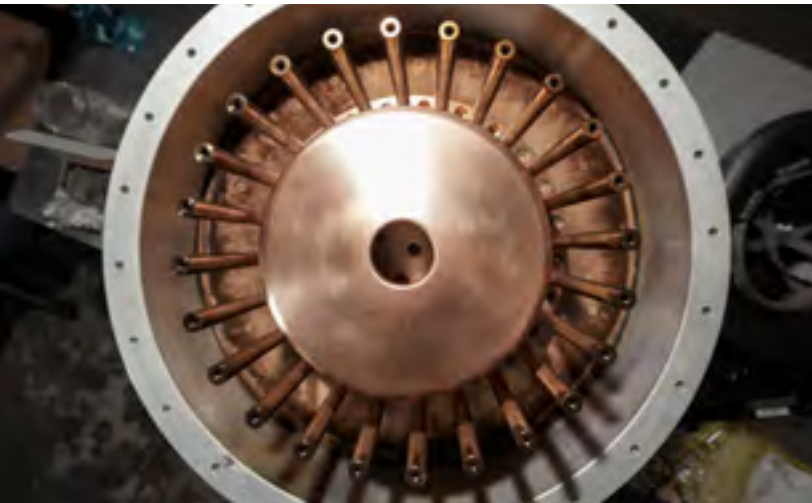
The length and shape of the anode and cathode, as well as other components of the DPF device, were designed to reliably produce the most neutrons possible based on hundreds of kinetic plasma simulations. (Photo by Garry McLeod.)
