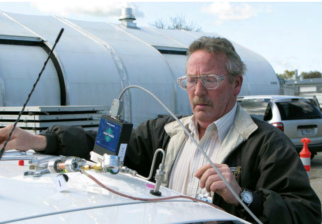
Above: Tim Ross draws a sample of hydrogen from an in-vehicle cryogenic fuel tank. The sample will be taken to Livermore's Raman spectroscopy lab to measure the ratio of para- to ortho-hydrogen. Below: The Raman spectroscopy apparatus. The sample container is visible in the center-right as a pair of brass-colored crossed pipes with a green knob.
