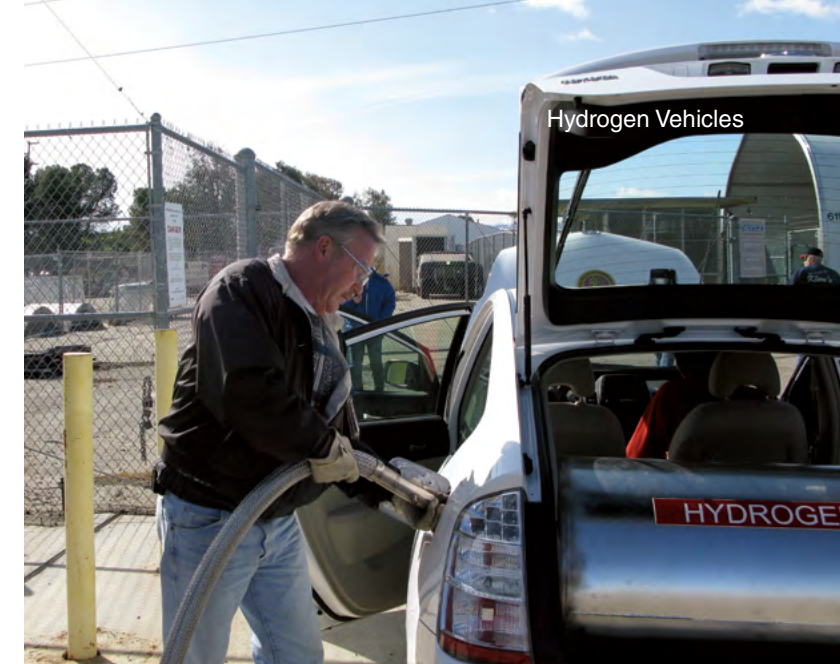
Retired Laboratory technician Tim Ross fuels up a cryogenic tank with hydrogen at the Laboratory's Cryogenic Hydrogen Test Facility.
