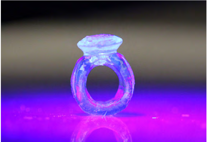
Livermore researchers can quickly 3D print stronger, more flexible objects from thiol-ene resins using CAL, a volumetric additive manufacturing (VAM) technology. (Photo by Maxim Shusteff.)
