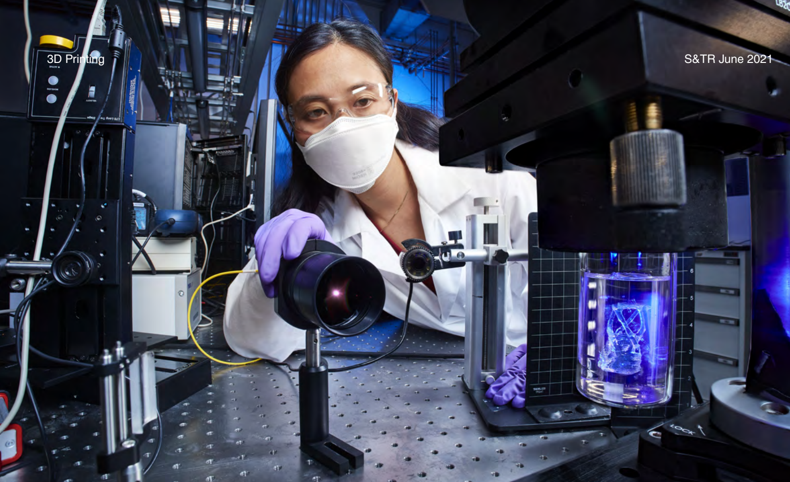
Livermore scientist Erika Fong demonstrates how CAL creates a three-dimensional, solid part within a container of resin. (Photo by Garry McLeod.)
