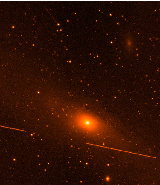
A composite false-color image of the Andromeda galaxy was created by stacking five wide-field-of-view channel images for an exposure of eight seconds. This image demonstrates the exceptional stability obtained by the Tyvak-0130 bus for a nanosatellite-class vehicle. During this series of exposures, two satellites moved through the field of view. Both are represented as two aligned streaks, with the bright set near the middle and the fainter and shorter streaks at left.
