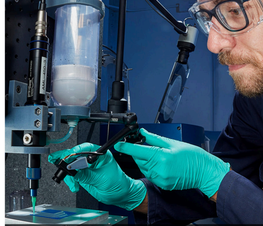
A researcher produces a test component using direct-ink-write additive manufacturing. LLNL is introducing new manufacturing methods into stockpile modernization programs.
