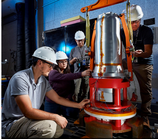
Engineers in the W80-4 LEP conduct environmental testing on a mock test unit to ensure systems will work when needed, but never when not needed.
